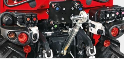
Modular hydraulic system with up to 11 hydraulic couplings divided into continuous flow, double acting and free return. All connections are served by hydraulic hoses with an increased cross-section to reduce pressure losses and thus improve the efficiency of the system.
