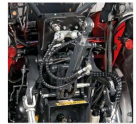
**HYDRAULIC LIFT ROD AND TOP-LINK\*** Allows the positioning and tilting of the implements to be corrected.
