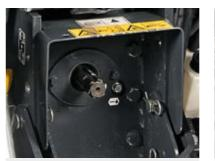
POWER TAKE-OFF Gearbox with rear PTO 540/1000 rpm
