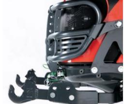
FRONT LIFT\* auxiliary device with adjustable arms and quick couplers complete with bullbar. The front lift allows combined use of front and rear implements.
