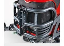
Tubular steel element to protect the bodywork; integrates the top link in the configuration with the front lift.
