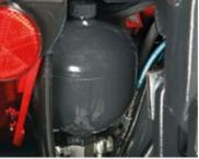
helps absorb jolting transmitted from mounted implements, thereby increasing driving comfort and protecting both machine and operator from potential harm.
