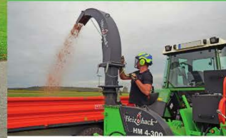
Discharge chute adjustment manually
