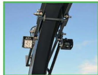
Camera and LED headlights placed at the discharge chute for best view
