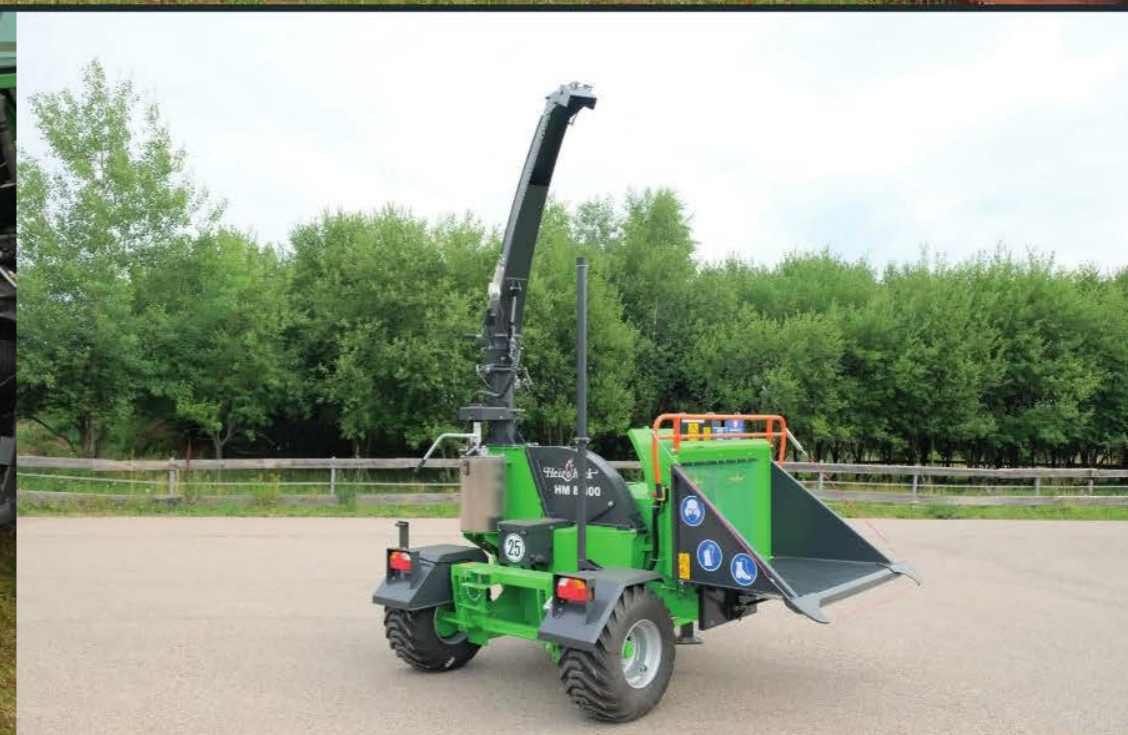
Discharge chute and flap electrical
