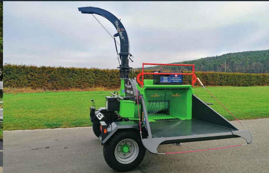
Discharge chute adjustment manually
