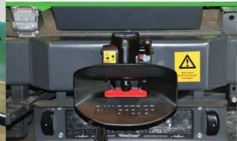
Automatic trailer coupling with compressed air connection
