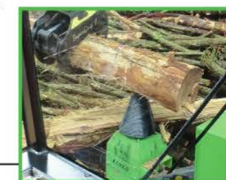
Cone splitter for pre-splitting of logs
