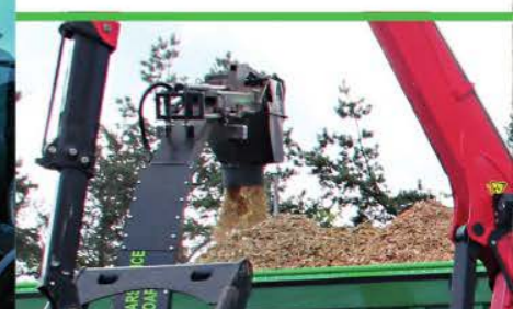
Cyclone for dust reduction
