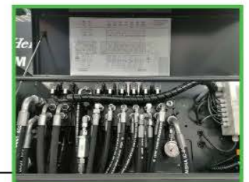
Hydraulic block incl. lever for manual operation
