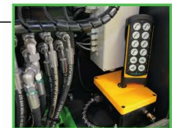
Radio remote control various hydraulic functions adjustable
