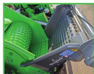
Conveyor belt at the Infeed table aggressive and powerful material infeed, can be used as a funnel
