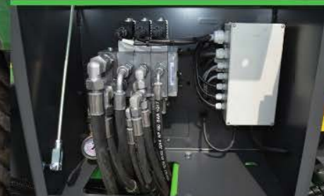
Hydraulic control block
