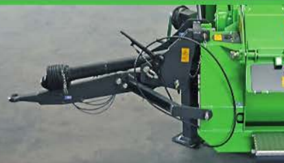
Hitch - height of towing port 500 mm
