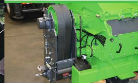
Massive V-belt transmission
