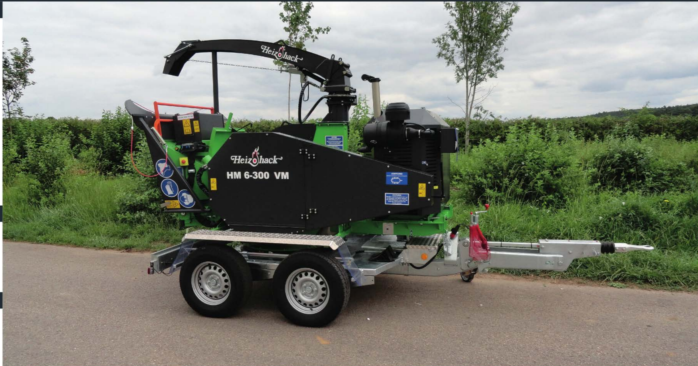
Massive turnable assembly 270° rotatable
