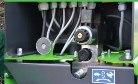
Speed of infeed adjustable by flow divider
