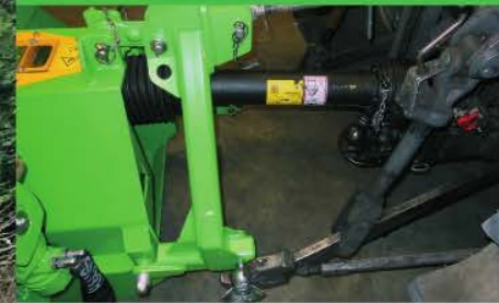
3-point-linkage extension with free wheel
