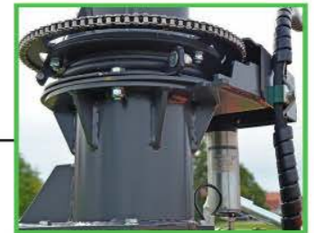
Discharge chute rotatable drive via electric motor
