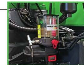
Automatic central lubrication easy and fast lubrication
