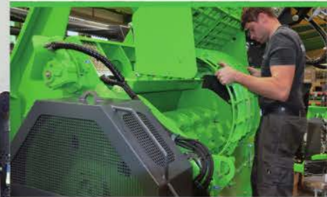
Multipiece sieve for easy exchange
