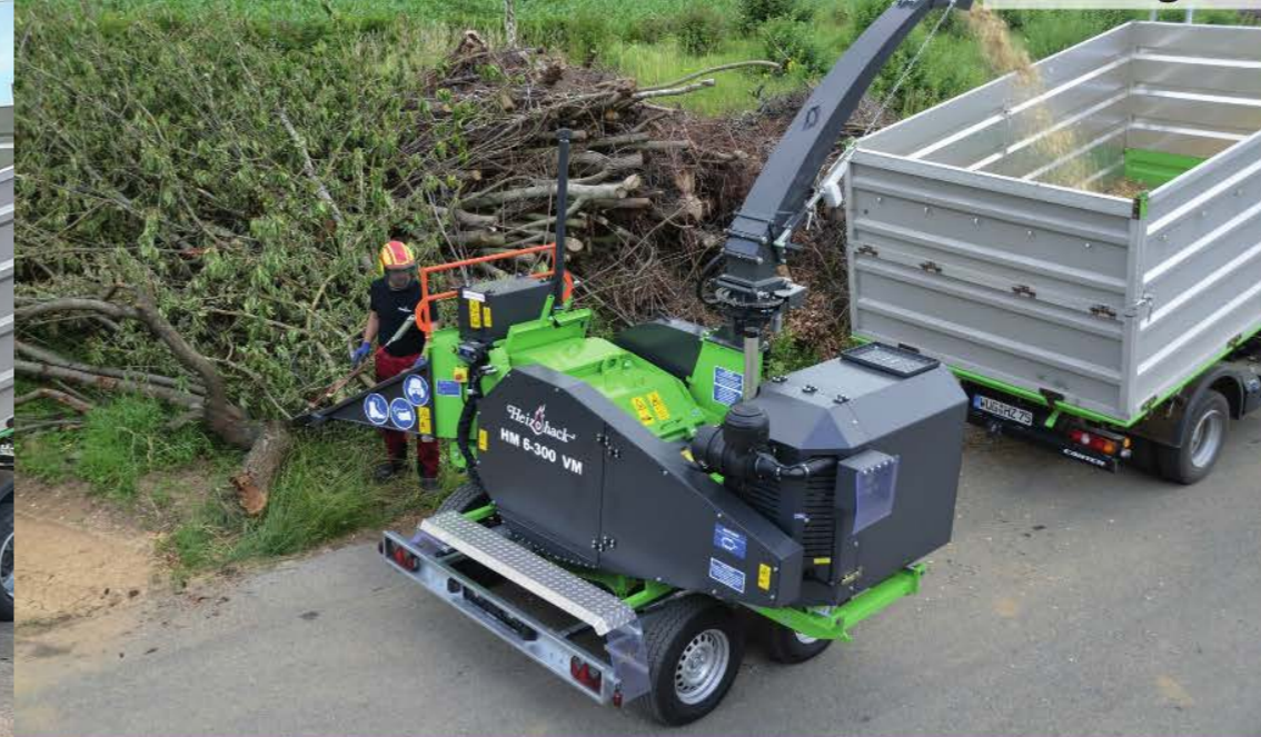
Height-adjustable drawbar with coupling ring or trailer ball
