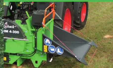
Infeed switch off due to safety rope from steel
