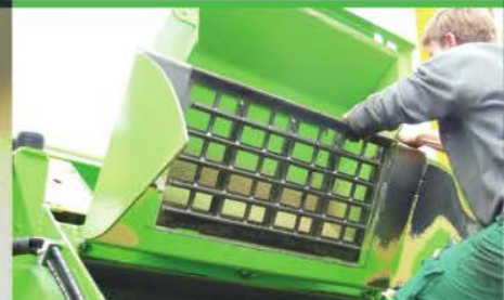
Rotor cover with extra sieve
