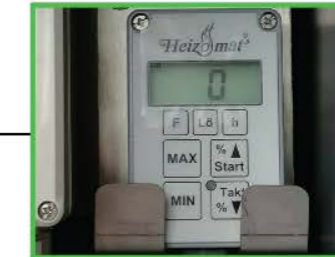
Speed-regulated Infeed anti-stress-control
