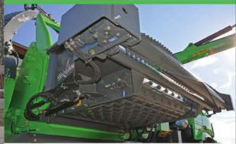
Front end roller with heavy hydraulic drive
