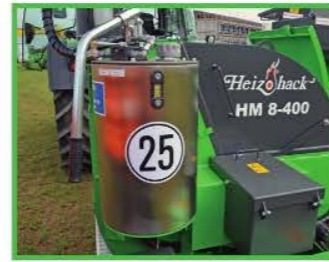
Height adjustable discharge chute with own oil supply hydraulically adjustable
