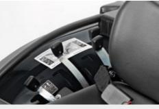
POWER LIFT Auxiliary rear hydraulic remotes with 3 distributors (2 double acting and 1 single acting), 1 oil reflow.
