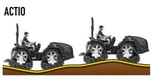
Thanks to the 45° offset of the front and rear axle final drives, the Mach 4 combines a long wheelbase with a reduced engine overhang: features which grant perfect stability in all operations, ensuring maximum safety and comfort at all times.
