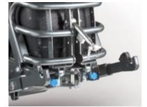
FRONT LIFT Used together with the bullbar and 1 double-acting distributor, it allows all the frontal equipment to be used.
