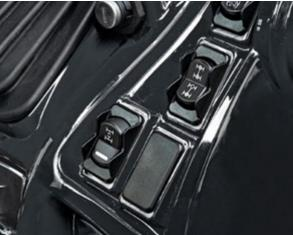
DIFFERENTIAL LOCKS CONTROL The front and rear differential lock prevents slipping and optimizes traction.
