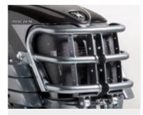
BULLBAR Tubular steel guard protecting the bodywork; integrates the third-point for the front lift.
