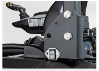
**EXTERNAL CONTROLS OF THE POWER LIFT UNIT\*** Raise and lower the rear power lift unit (with driver on the ground at the side of the machine) during hitching of the carried interchangeable tool.
