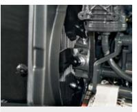
ACS (Automatic Clean System) Engine cooling fan with air flow reversal. Reduces the need for cleaning the front grille, ensuring more constant engine cooling.
