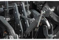
**RAISED 3-POINT HITCH\*** For a lifting geometry favourable to the adjustment of the implements.
