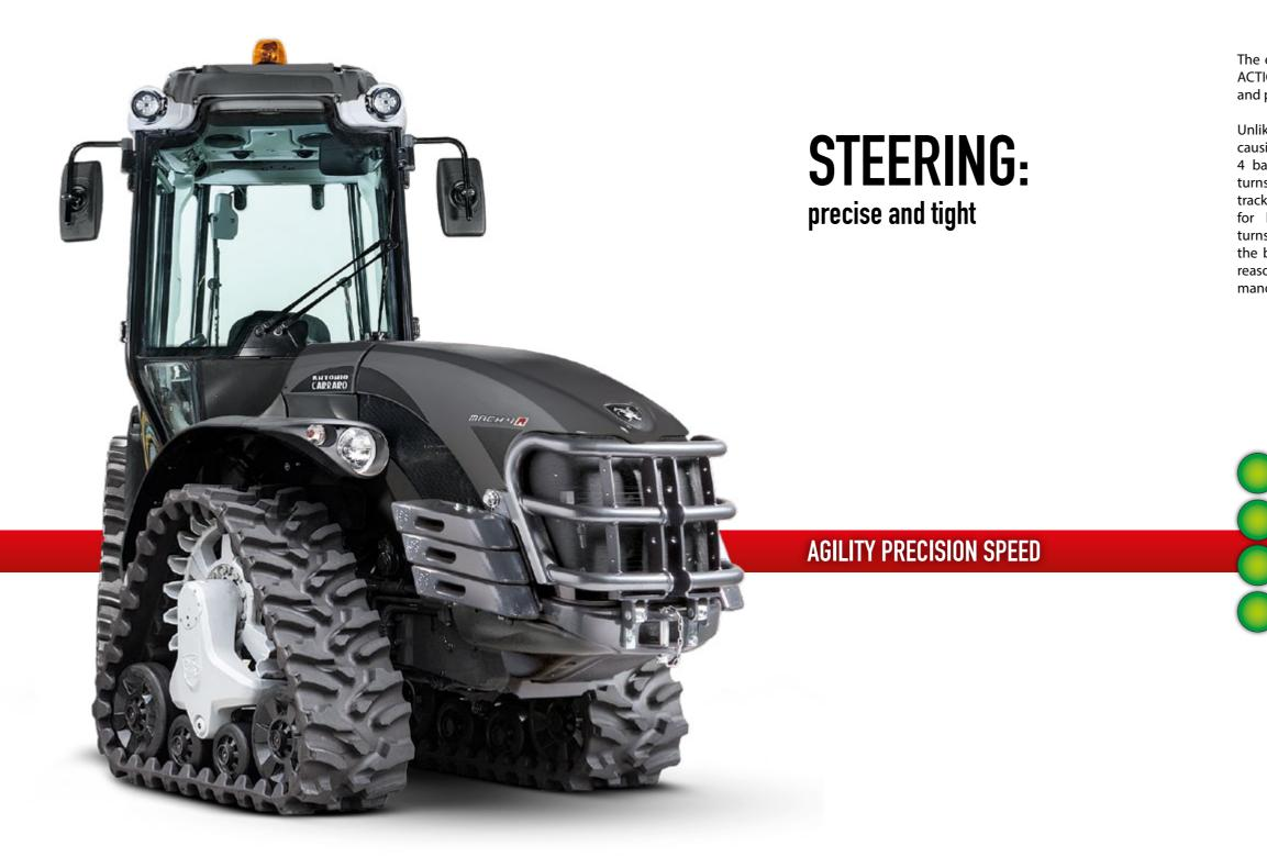
The extraordinary agility of Mach 4 results from the ACTIO<sup>™</sup> articulated chassis which allows tight turns and precision manoeuvres in confined spaces.
