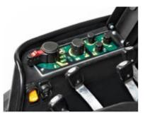
ELECTRONIC LIFTING Electronic lifting at controlled position and effort with damping for road transfer.
