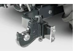
**3-POINT LINKAGE** Adjustable lifting arms with Cat. 2 and Cat. 1\* quick coupling with adjustable width.
