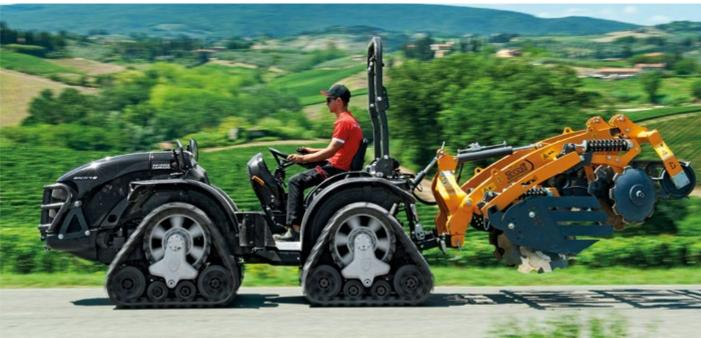
The "floatation" of the vehicle on the ground surface allows for excellent use of Mach 4 all year long, making it possible to work on wet, muddy, marshy, crumbly, snowy and sandy terrains. The perfect weight distribution on the rubber track treads makes for minimum compaction, inferior to that of footprint.
