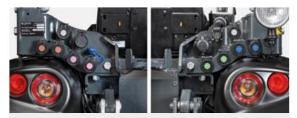
HYDRAULIC SYSTEM Electro-proportional hydraulic system controlled by joystick with double driver safety system and integrated control unit with user-adjustable settings - 12 rear quick couplings. External lifting control.
