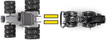
The four alternate-grip rubber tracks (w: 35 mm / 1,37 in), similar to "ground profile" tyres, assure constant adherence during all manoeuvres, even on slippery ground.
