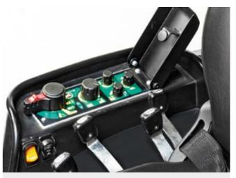
**ELECTRONIC LIFT CONTROL\*** Electronic position and draft control of the linkage with integrated maximum lifting height, rate of drop and damping control. Located in a control console including a lid that can be opened.
