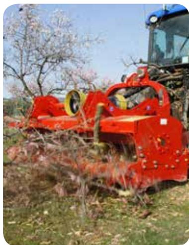
Certain crops produce very high quantities of prunings. This can cause big problems when it is time to mulch them. Burning is always bad for the environment. The MINIFORST pick-up provides a perfect solution – picking up the prunings with a pick up reel at ground level and, if needed, reinforcing the feed into the machine with an optional top reel. The prunings are then processed within a screen to produce a fine and uniform mulch.
