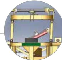
3-point linkage with spring tension and parallel-linkage side shift
