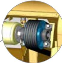
belt transmission with spring tension and safety coupling
