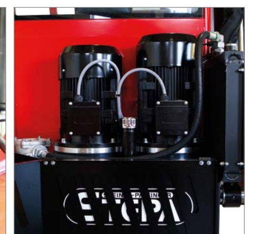
optionally with two electric power units
