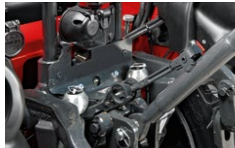
REAR AUXILIARY ACCESSORIES Top link attachment, lift arm ball housing, 7- and 3-pole electrical sockets.
