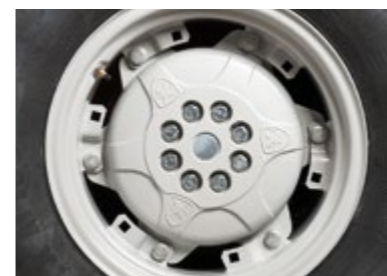
REAR CAST IRON WHEEL FLANGES Flanges that increase the weight of the tractor at the rear.
