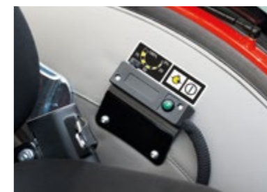
CONTINUOUS FLOW SETTING* Proportional electrical control for setting continuous oil flow up to 50 l/min.
