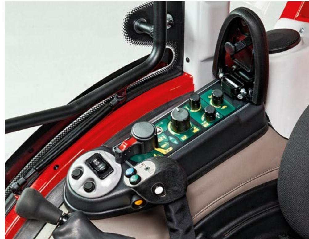
ELECTRONIC LIFT CONTROL* Electronic position and draft control of the linkage with integrated maximum lifting height, rate of drop and damping control. Located in a control console complete with opening armrest cushion.
