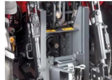
SLIDER HOOK Integrated into the rear lift, it gives the operator various options for the practical setting up of the tractor and the rapid alignment of the towed equipment.
