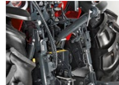
VERTICAL TIE-ROD AND HYDRAULIC THIRD-POINT Optimizes the positioning and inclination of the equipment.
