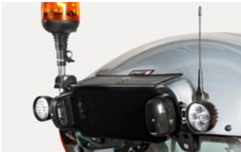
LED rear work lights, licence plate holder and folding support for flashing beacon.
