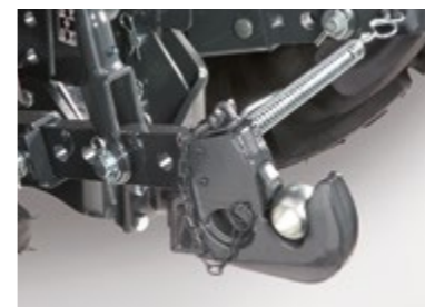
ADJUSTABLE BARS Rear 3-points linkage with adjustable bars and quick couplings.
