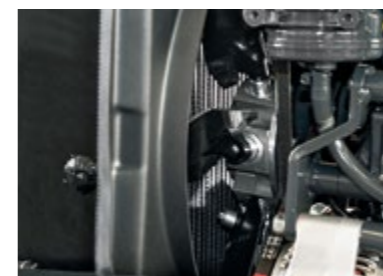
ACS (Air Clean System) Engine cooling fan with air flow reversal. Reduces the need for cleaning the front grille, ensuring more constant engine cooling.
