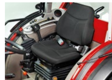
PNEUMATIC SEAT Latest generation with air springs.
