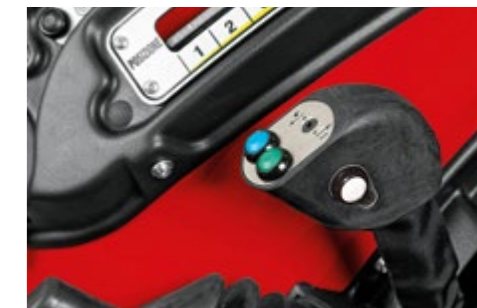
HAND GRIP WITH ELECTRICAL CONTROL BUTTONS Controls for proportional activation of the remote valves.
