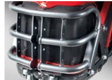
BULLBAR Tubular steel guard protecting the bodywork; integrates the third-point for the front lift.
