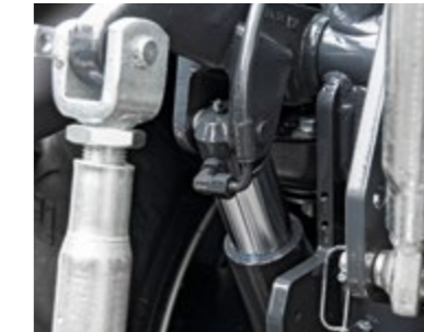
HYDRAULIC SUSPENSION Hydraulic suspension on the UNIFLEX rear powerlift.
