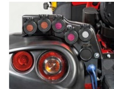
REAR QUICK COUPLINGS Electro-proportional hydraulic system controlled by joystick with double driver safety system and integrated control unit with user-adjustable settings - 12 rear quick couplings.
