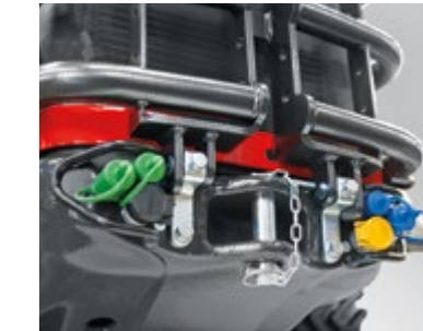
FRONT QUICK RELEASE COUPLINGS Front powerlift > 6 couplings replicated on the rear, of which 2 with double effect + 1 electronically adjustable continual delivery and 1 simple effect.
