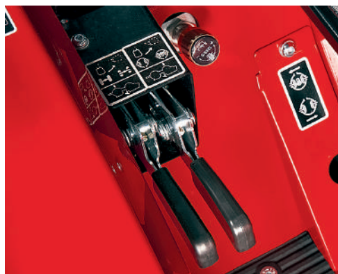
DIFFERENTIAL LOCK AND DRIVE DISENGAGEMENT
